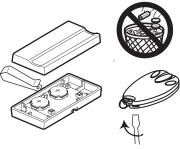
To replace cover, snap shut along both sides. The lithium batteries should produce power for up to 5 years. To replace batteries, use a coin, the visor clip or screwdriver blade to pry open the case, as shown ("Open" location is stamped on back.)
